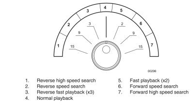
Figure 23. Direct Shuttle Ring Speed Settings
